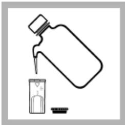
17. Immediately empty the sample cell. Rinse the sample cell and cap three times with deionized water.
